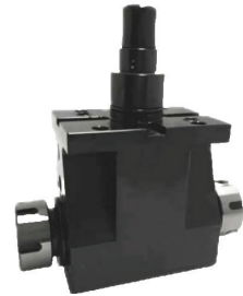
Universal driven toolholders 4500~12000rpm Adjustable angle of \pm 90 degree
